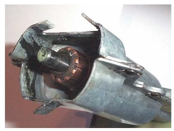
The commutator is the key at this point. If the commutator looks very blackened and pitted after cleaning, or if the wiring on the armature looks heavily burned, you may have a motor that is not repairable. That is not very common, but does happen. If you find the brushes are O.K. and need to replace the motor, you haven't lost anything but time.
