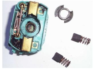
Remove the end cap carefully to avoid losing any of the small parts that may fall and disappear into the dark recesses of the door. The cap contains two carbon brushes, which may be almost non-existent, two brush springs, and a flat/round brush retainer. There will also likely be a lot of carbon dust inside the cap and motor housing, along with the remnants of the original lubricating grease.
